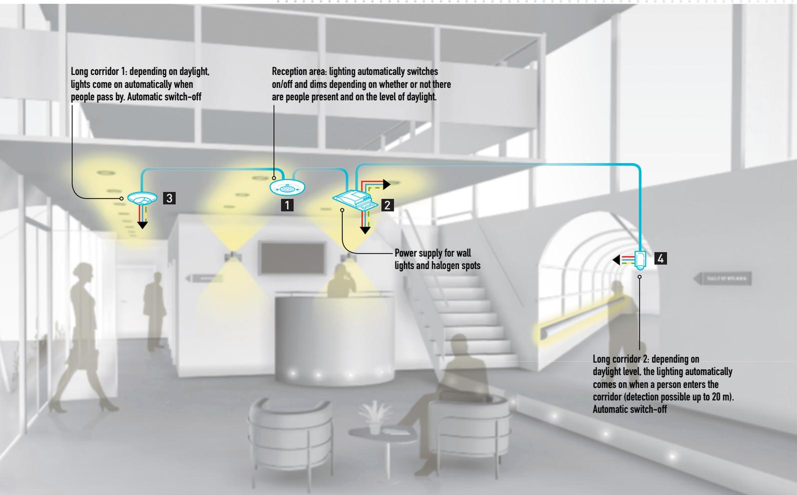
Long corridor 1: depending on daylight, lights come on automatically when people pass by. Automatic switch-off
